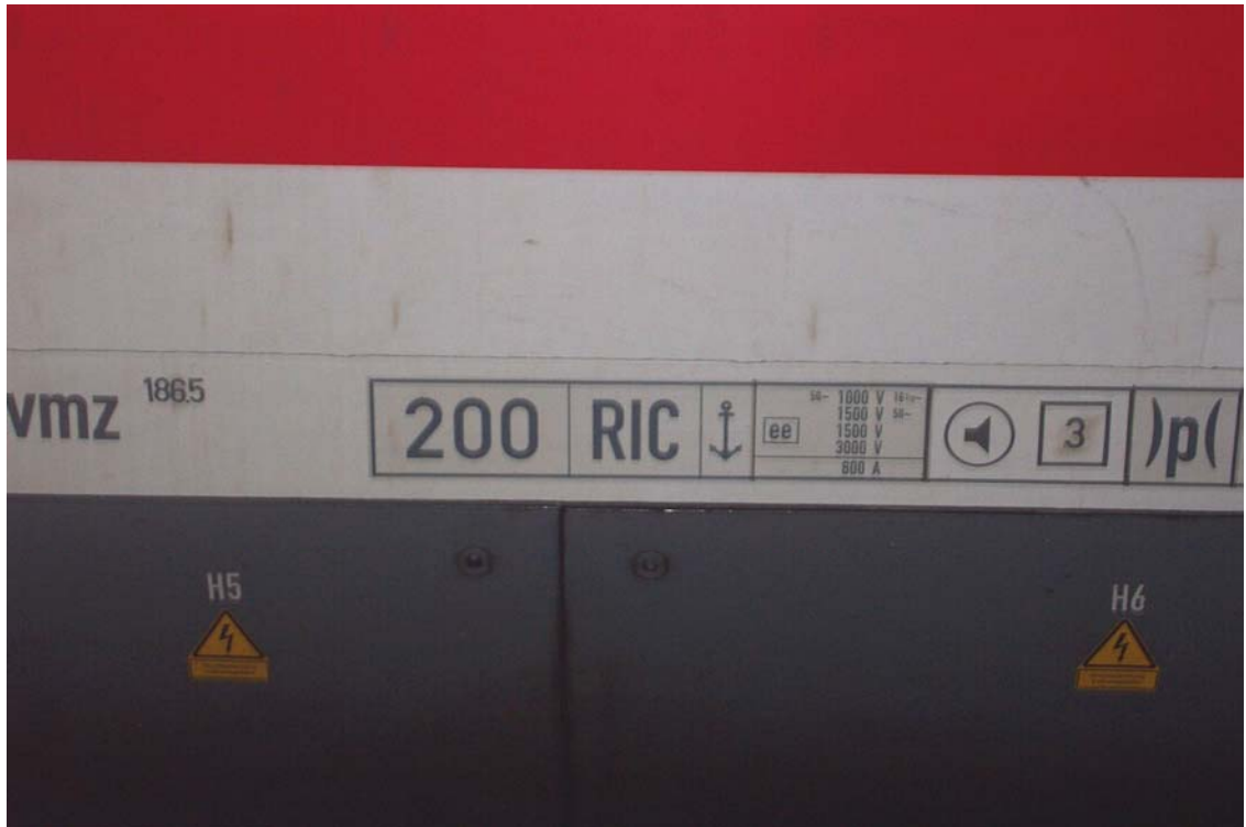
Figure 9 - UIC Markings on Conventional European Intercity Coach
